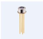
The OTP-628D2 is a thermopile sensor in classic TO-46 housing. The sensor is composed of 116 elements of thermocouple in series on a floating micro-membrane having an active area of diameter 545  $\mu\text{m}$ . The thermopile sensor provides nearly Johnson-noise-limited performance, which can be calculated by its ohmic series resistance. A thermistor with a lead connected to ground is also provided inside the TO package for ambient temperature reference.
